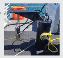
to be installed or removed quickly even when towing operations are underway, without the use of tools. Constructed in corrosion resistant and durable aluminium and stainless steel, Webtool™ cutters can be easily integrated into existing vessels or systems and do not cause chaffing or premature wear of the towline.
