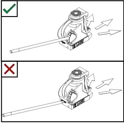
Figure 5 – Manoeuvring the Jack
