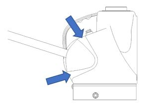
Figure 1 – Pinch Points on the Jack
