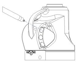
Figure 7 - Inserting the Operating Lever
