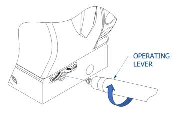
Figure 6 - Tightening the Release Valve Screw
