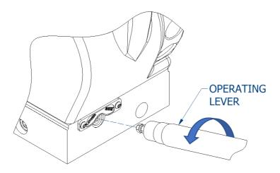
Figure 9 - Closing the Release Valve Screw
