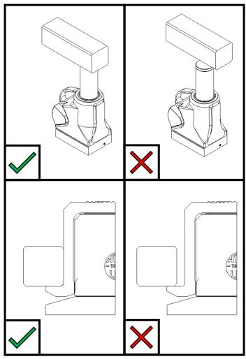
Figure 4 – Applying Loads
