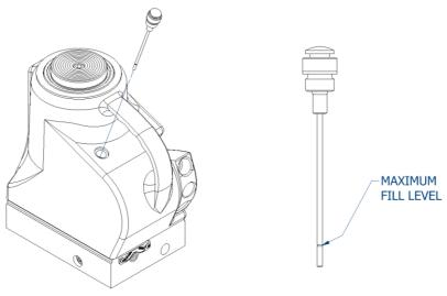
Figure 2 – Removing and Checking the Dipstick
