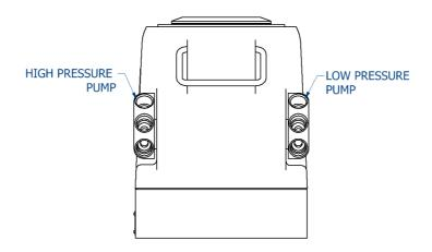
Figure 14 – High and Low-Pressure Pumps
