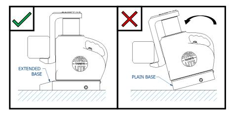
Figure 13 – Always Use an Extended Base with a Claw
