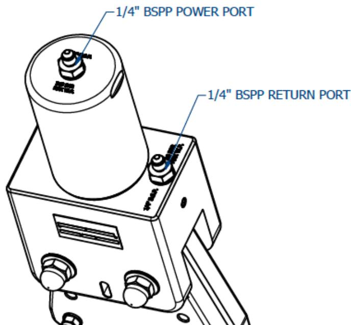
Fig 1 – Hydraulic connection points.
