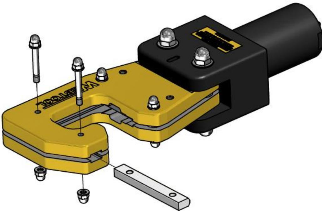
Fig 5 – Removing the anvil
