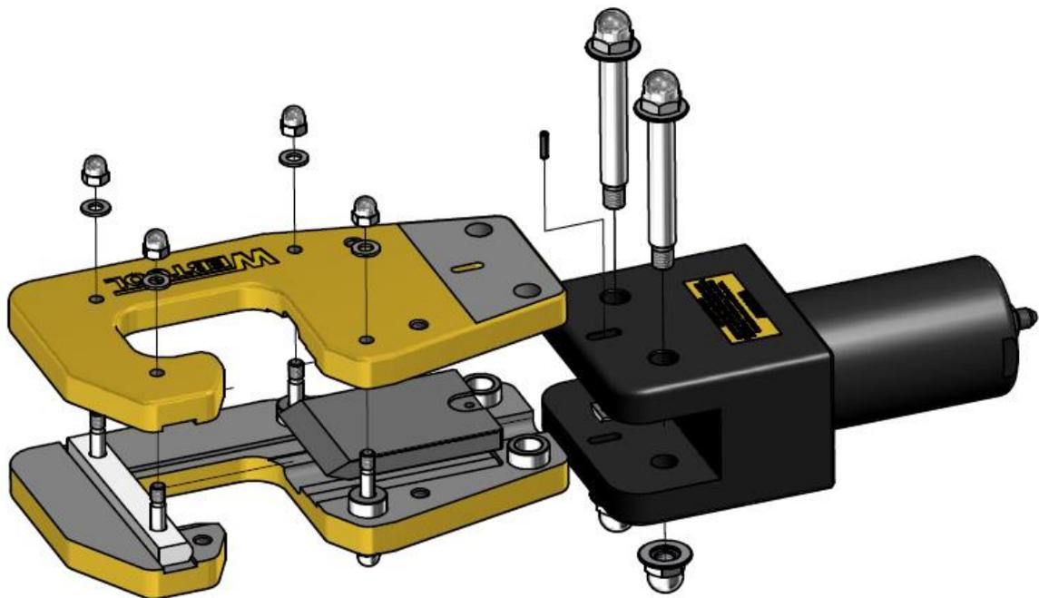
Figure 4 – Removing the blade
