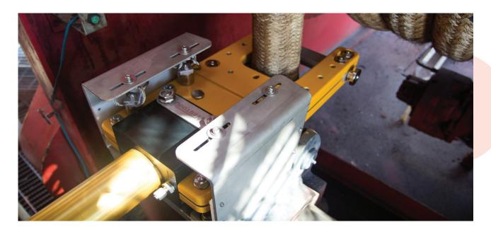
**Winch line cutters**, designed and manufactured by Allspeeds, are an essential element in contingency planning for many maritime, subsea and offshore applications. The steel wire and fibre rope winch line hydraulic cutters provide an immediate cut in the event of difficulties that put personnel, vessel and project delivery at risk.
