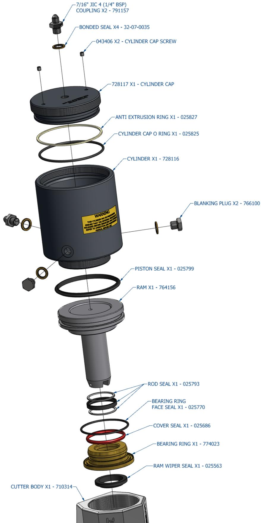
**4.5.2 View of Internal Components in Assembled State**
