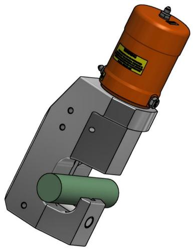
Operate the main ram power port to sever the wire rope, hold pressure until the wire rope is severed. Once the wire is severed, pressurize the main ram retract port to withdraw the cutting blade. Do not try to remove the anvil when the blade is fully extended. If a further cut is required, the above procedure should be repeated.
