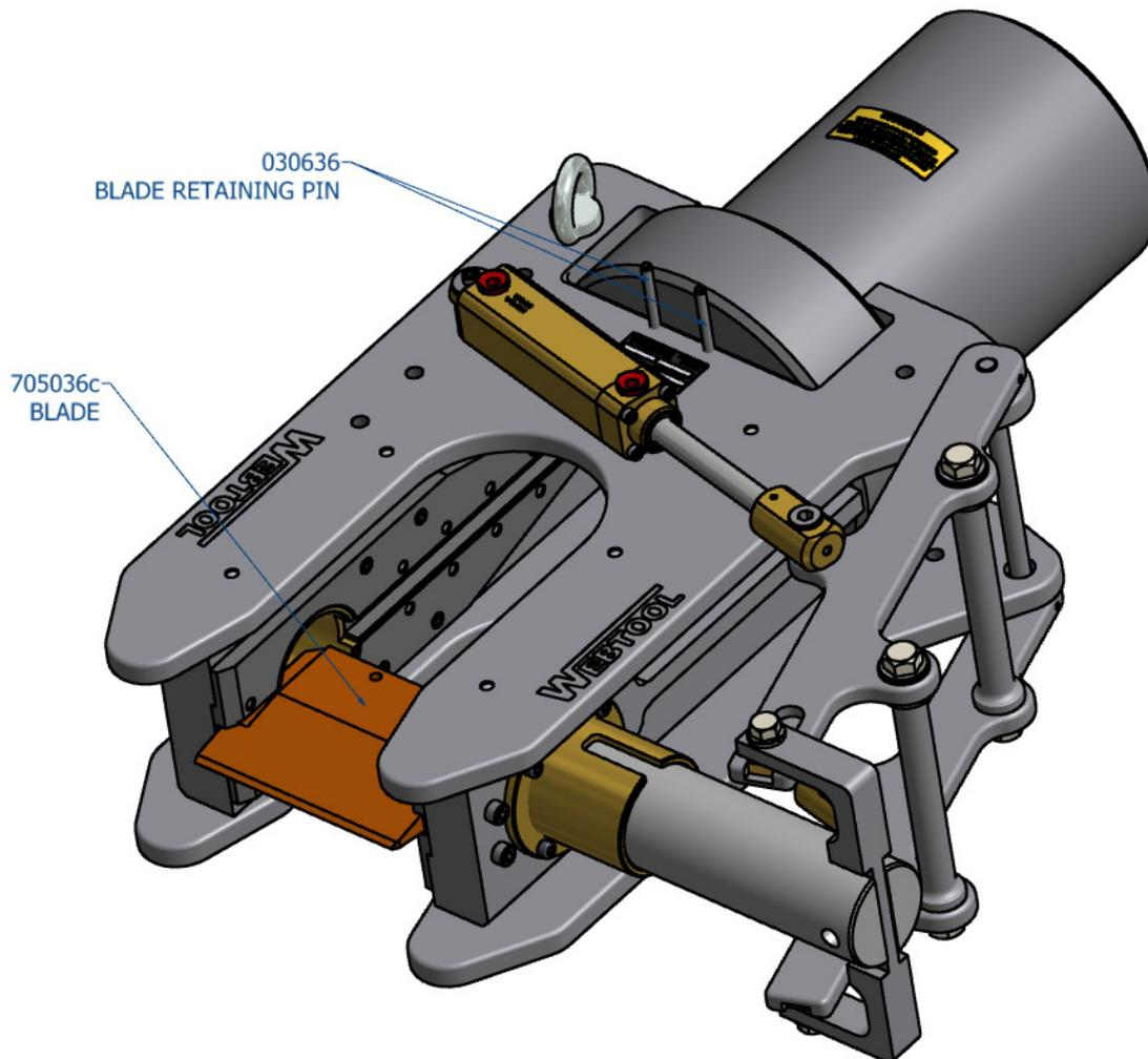
With the pins removed the blade can be taken from the cutter, gloves should be worn to prevent cuts from any sharp edges that may be present on the blade after use. Re-assembly is the reverse of the above process.
