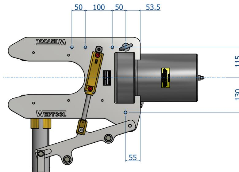
Two hydraulic supplies are required, ported as shown below. The maximum working pressures are shown in the table below and pressure limiting valves must be fitted into the supply to limit the pressures to these levels. The weight of the tool is 125kg.
