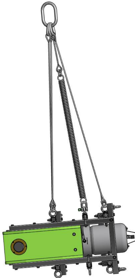
Figure 25 – RCV215A not level
