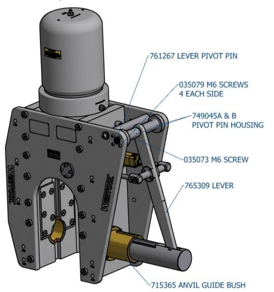
Withdraw the pivot pin 761267 far enough to release the lever arm. (There is an M6 tapped hole in the end of the pivot pin to assist in withdrawing this) The lever arm can be moved upwards to separate it, with the anvil pin 761247, from the anvil SSC6500. The anvil may now be slid out from the anvil guide bush. Re-assembly is the reverse of the above process.
