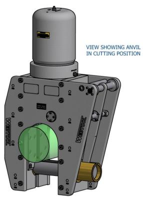
Operate the main ram down-stroke to sever the wire rope. Once the wire rope is severed, Pressurize the main ram retract port to withdraw the cutting blade. Then, and only then, retract the anvil. It is important not to operate the anvil cylinder whilst the main ram and blade are in the fully extended position.
