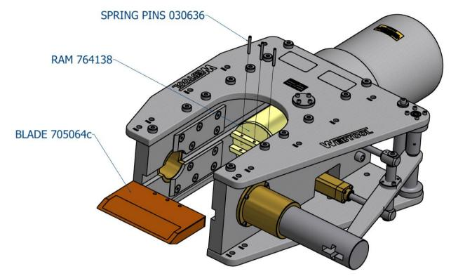
With the pins removed the blade can be taken from the cutter, gloves should be worn to prevent cuts from any sharp edges that may be present on the blade after use. Re-assembly is the reverse of the above process.
