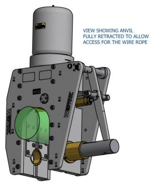
Operate the auxiliary cylinder instroke to position the anvil fully home under the wire rope, the main ram should not be activated until the auxiliary cylinders are operated to the full extent of their stroke.
